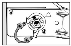
Using adjustable pliers, pull out the retaining clips on the right and left of the support plate.
